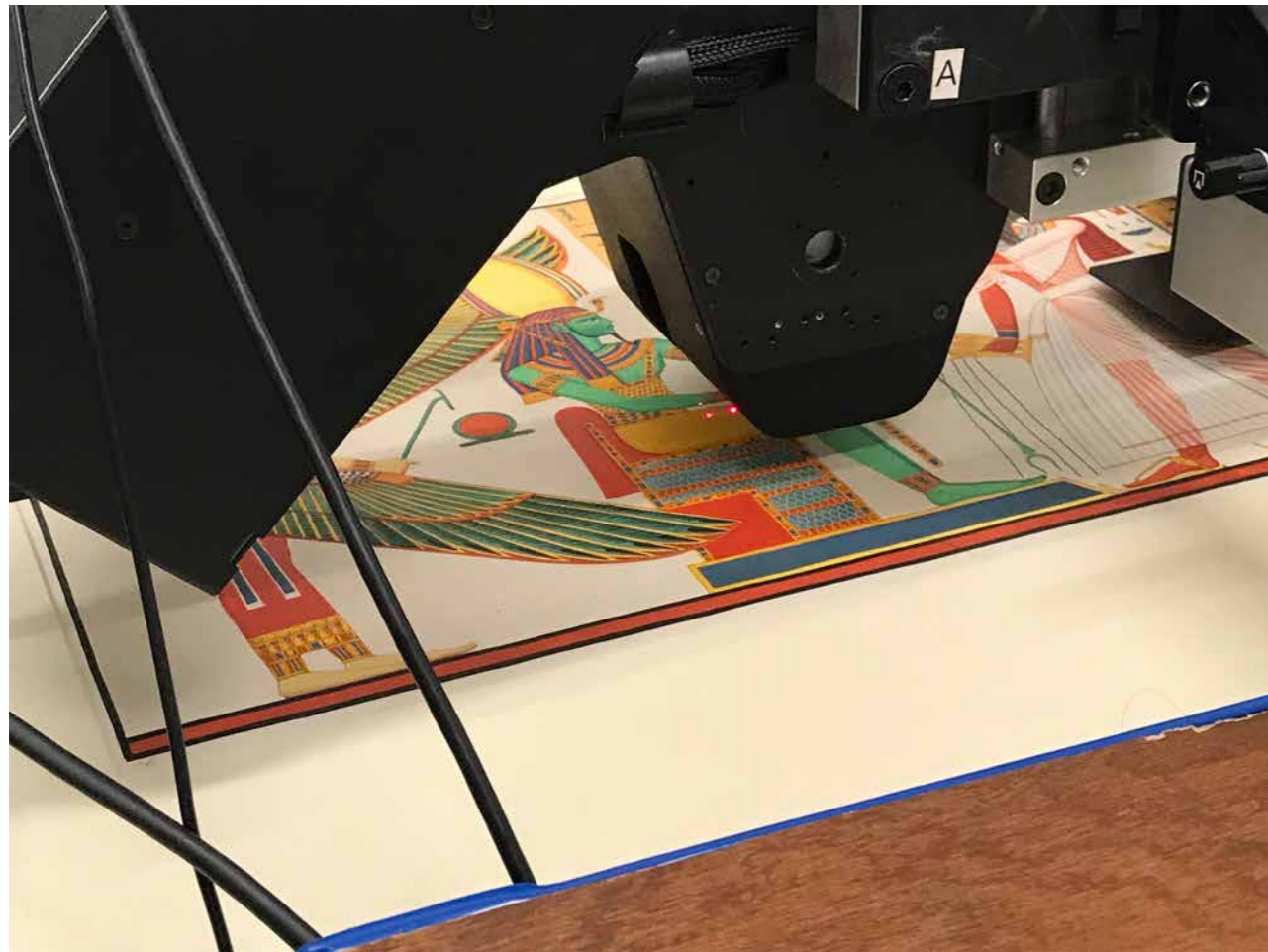
Below: Analysis of a work from John Ruskin's teaching collection using the Hydra (combined XRF/XRD)
